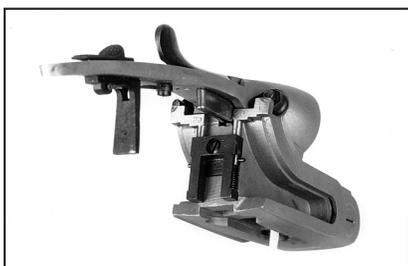
An automatic safety mounted on the top tang is engaged when the top latch lever is pushed to the right. Pushing the safety button forward disengages the gun's safety.
