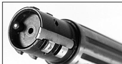
The new Mark V Lightweight's bolt still bears unmistakable Weatherby touches, such as its claw extractor, fluted body, three gas vent holes and distinctive bolt shroud.
