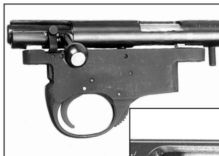
**A massive, matte black, non-ferrous metal casting serves as the Woodchucker's trigger housing. The assembly also contains the trigger group, magazine and magazine release. One piece serves as both the ejector and bolt guide. The steel part is screwed into the gun's receiver and has upward extensions that correspond to grooves in the bolt.**
